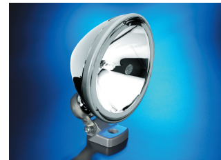
Comet 200 Chromium – IAM 007 893-191 H: 153 mm W: 76 mm D: 144,5 mm Exclusive chrome styling / Classic stylish outfit / Clear-glass design / FF high-gloss reflector / Aluminium vapour-coated reflector
